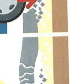
surface into the hole collapses the road Weight of traffic water creating a hole Sun dries up the under the road
